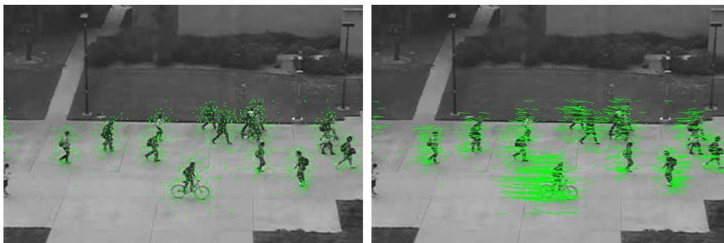
Figure 3.1: The pictures above were taken from UCSDped2, Test002 video at frame 150. The first picture visualizes the feature points (green points). The second picture visualizes the feature point trajectories (green lines).
